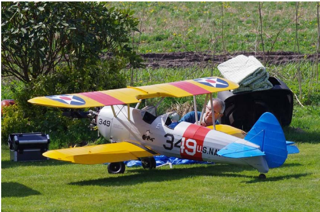
Note the elevator and U/C damage as Tony assesses the condition after recovery.
