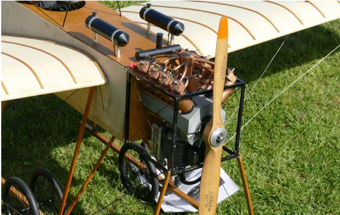
I'm advised that the octopus like contraption on top of the engine is the water cooling system for the V8 engine of the original aircraft!
